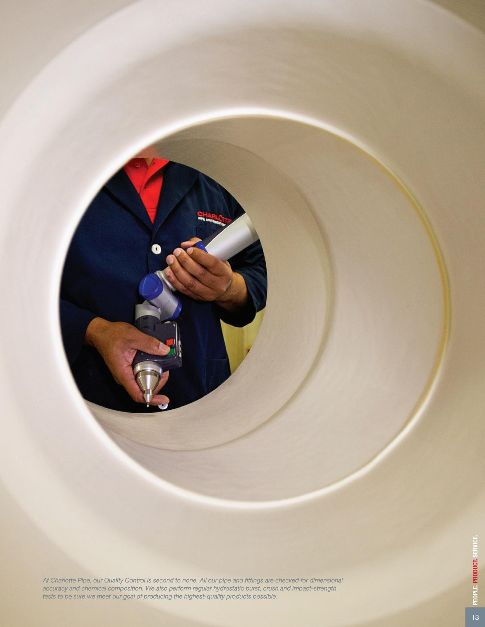
*At Charlotte Pipe, our Quality Control is second to none. All our pipe and fittings are checked for dimensional accuracy and chemical composition. We also perform regular hydrostatic burst, crush and impact-strength tests to be sure we meet our goal of producing the highest-quality products possible.*
