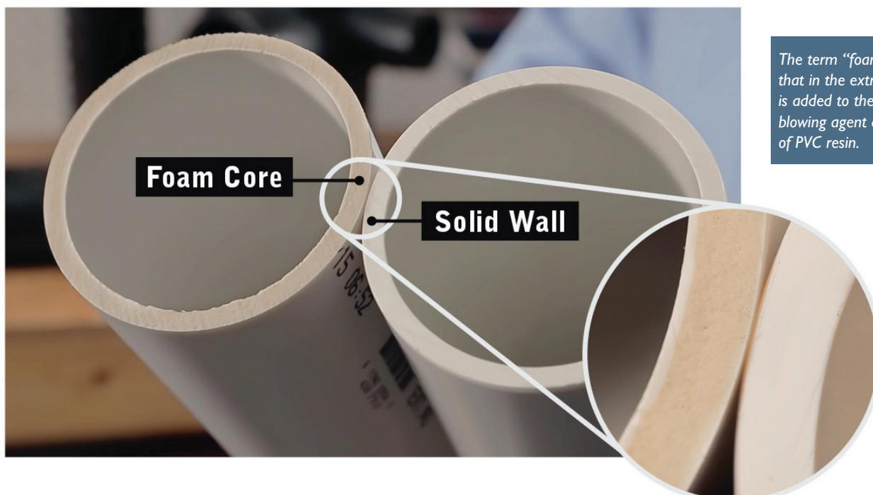
The term “foamed core” refers to the fact that in the extrusion process, a blowing agent is added to the PVC in the center layer. This blowing agent displaces a significant amount of PVC resin.
