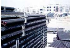
Cast-iron piping is a cost-effective solution when dealing with fire-resistive construction because it will not melt or burn away in a fire.
