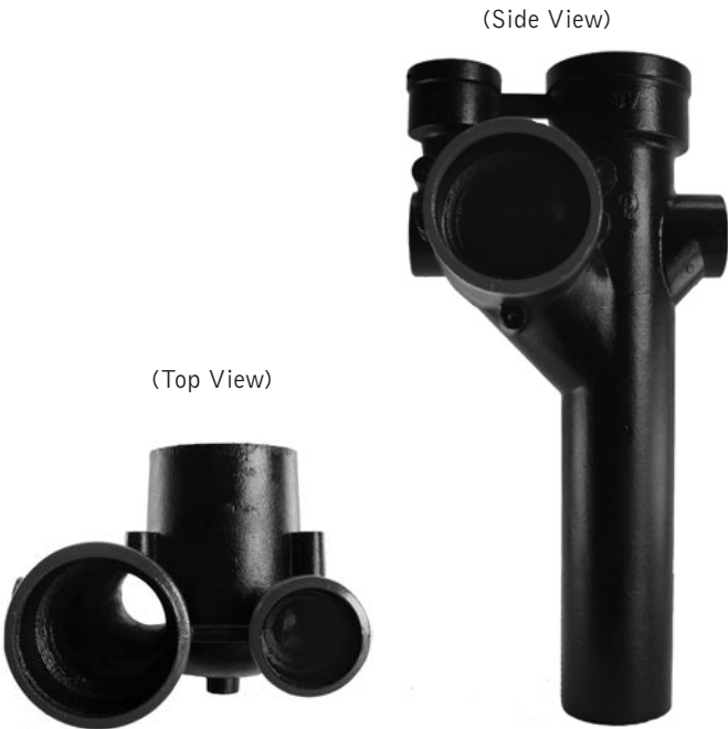
PART NO. SV 974L Left Hand Starter Fitting with 4" Hub and 2" Tapped "A" Side Inlet [Designed for use below or in the floor with bottom-outlet water closets]
