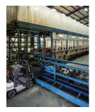
Charlotte Pipe's ecoating is an extremely efficient process for the application of coating onto a metal surface. Fittings and five-foot pipe lengths are sent through a 15-stage process, including multiple cleaning stages, followed by the application of a zinc phosphate base coat, and then two stages where a top coat is applied. The coating is then cured for one hour at 400 degrees F. An aesthetic improvement, ecoat offers customers a consistent, thin, even coating.
