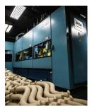
We continuously reinvest in our plants and equipment to be sure we are operating the most advanced production technology available and have the capacity required to fill orders completely and in a timely manner. We use automated high-volume equipment, like our Disamatic vertical molding machines, to produce our fittings at a rate of hundreds of molds per hour.
