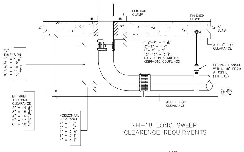
NOTE: RESTRAINT IS REQUIRED ON ALL PIPE 5" AND LARGER AT ALL BRANCH TAKE-OFFS, AND CHANGES IN DIRECTION TO PROTECT AGAINST HORIZONTAL MOVEMENT AND JOINT SEPARATION
