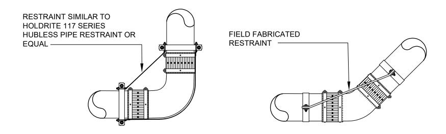
HORIZONTAL PIPE AND FITTINGS 5" AND LARGER SHALL BE SUITABLY BRACED TO PREVENT HORIZONTAL MOVEMENT. THIS MUST BE DONE AT EVERY BRANCH OPENING OR CHANGE IN DIRECTION BY THE USE OF BRACES, BLOCKS, RODDING OR OTHER SUITABLE METHOD, TO PREVENT MOVEMENT OR JOINT SEPARATION. THIS BRACING MAY BE FIELD FABRICATED OR A MANUFACTURED SYSTEM. THE DETAILS SHOWN ON THIS PAGE ILLUSTRATES SEVERAL METHODS OF BRACING.
